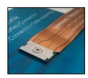
The FPC features gold-plated pads and integrated stiffeners on both ends and is secured to the X-Beam™ connector with a simple, highly reliable screw-down fastening system. By combining the advanced FPC design with an extremely short electrical termination path, these assemblies can uniquely combine high-speed signaling (>10Gbs) and significant power delivery (>5A). The XFPC Jumpers can be designed for signal, power or signal+power applications.
