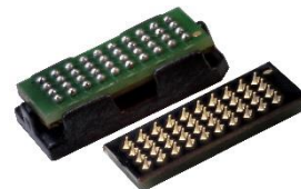
S310/311 - 40 pos LGA/BGA Connector
